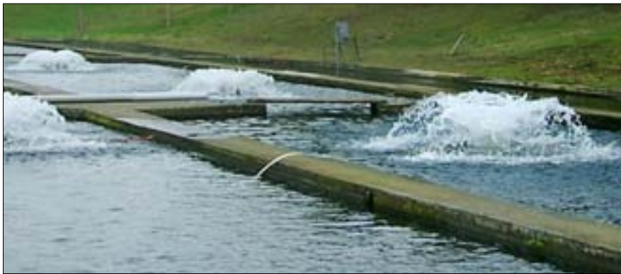
FLOBULL AERATORS in a trout raceway.
