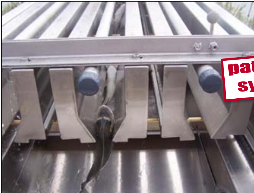
900gr sea bream in a Helios 50, view in the grading channels.
