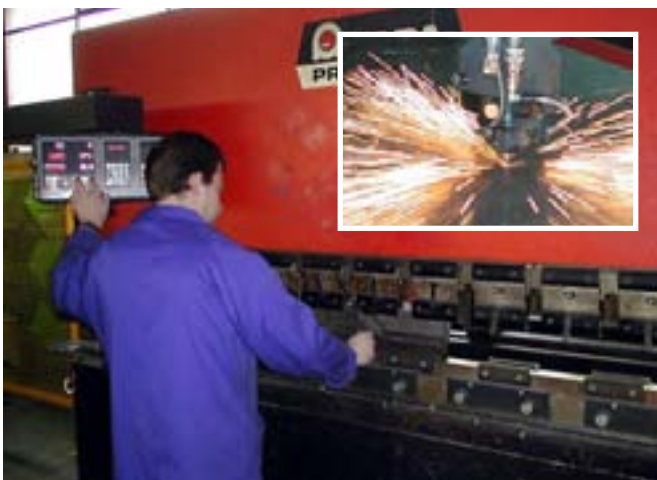
Digital controlled sheet working machine, and laser cutting is used to get the most complex shapes in stainless
