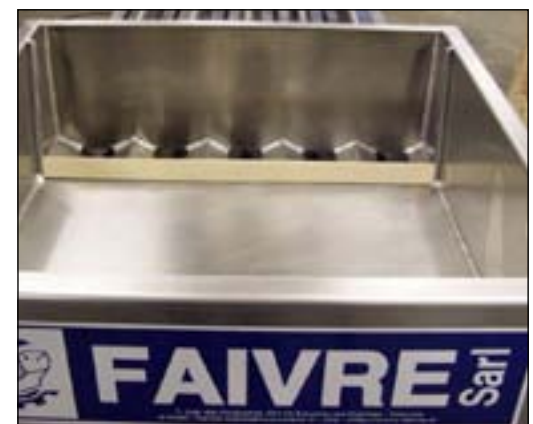
Inlet hopper with special system for Alevin.
