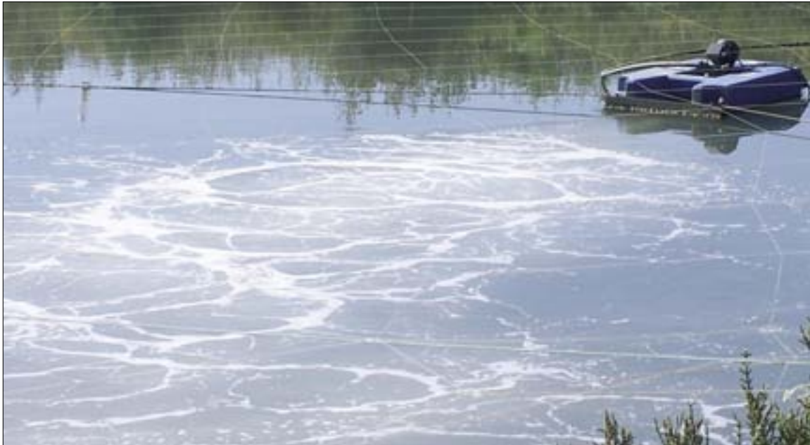
2 HP hydro-ejectors in a sea bass fish farm
